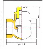
Test Pressure (Hydraulic) Shell : 1.5MPa Seat : 0.25MPa
