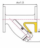
Test Pressure (Hydraulic) 35.15kg/cm²g (500psig) Working Pressure (Steam) 17.58kg/cm²g (250psig) Max. Working Temperature 225°
