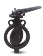
Intervalve® Butterfly Valve model IVGE / IVTLE is an economical answer to the corrosion problems faced by Chemical process industries with conventional metal seated Butterfly valves. The valve's unique design totally eliminates media contact with any metallic surface of the valve. The valve has a fully rubber lined body and a rubber encapsulated disc with a square slot for the drive end shaft.
